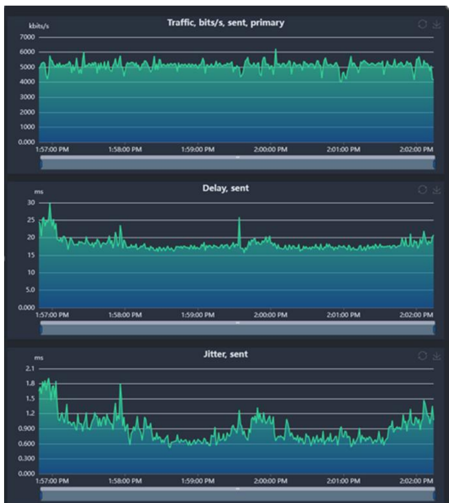
Figure 73 : UL KPIs for 5 Mbit/s RTMP video measured using Qosium
