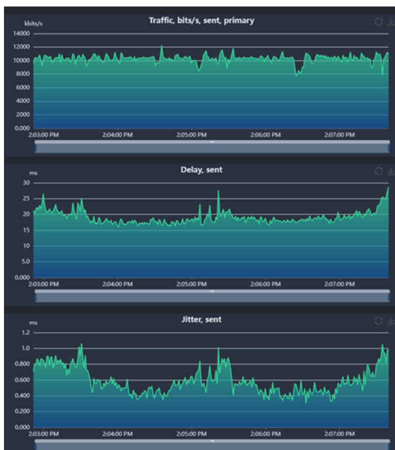
Figure 74 : UL KPIs for 10 Mbit/s RTMP video measured using Qosium
