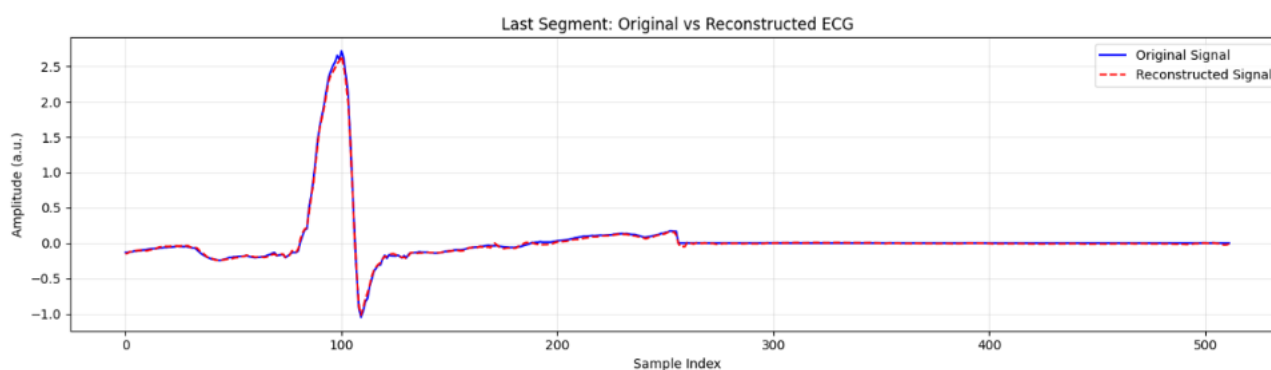
Figure 47 : Original and reconstructed signals for one beat starting with P wave at the output of the U-Net autoencoder
