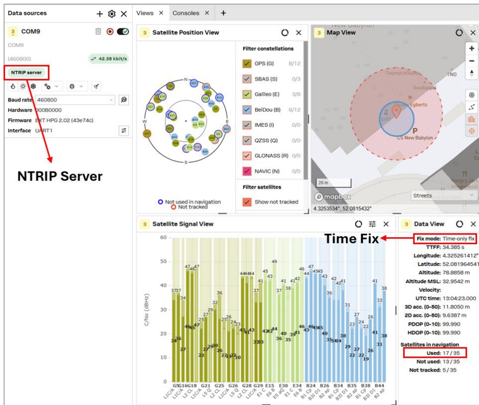
Figure 42. u-center-2 GUI for the base station configured as an NTRIP server.
