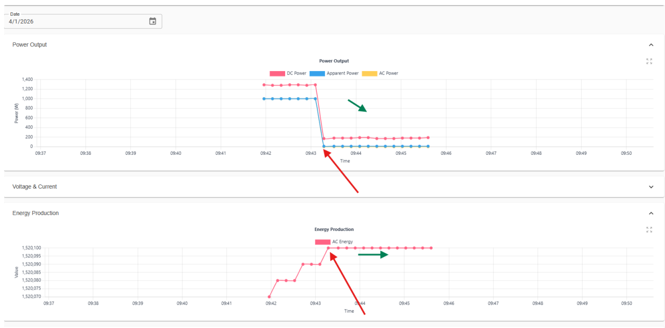
Figure 59. Inverter power limitation/increase effect.
