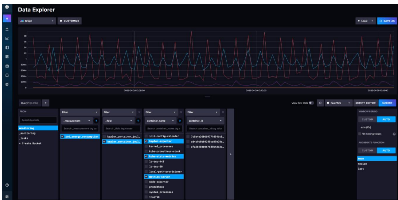
Figure 33: The InfluxDB data storage, part of the Monitoring Platform, which is collecting energy consumption data from k8s-based services
