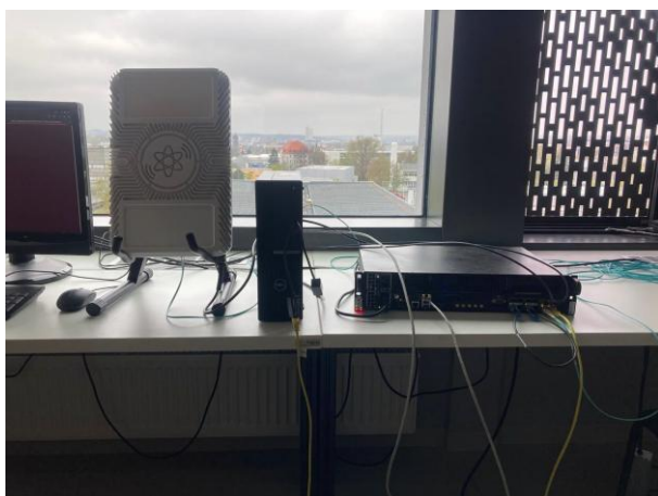
a) Overall setup view (CellBox Air radio unit and RAN server)
