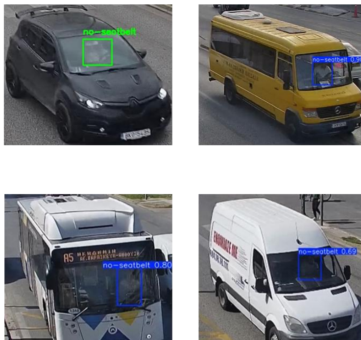
Figure 57: T5 AI functionality for incident detection (preliminary/indicative results pre-trial)
